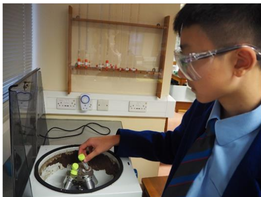
Centrifugation at 1000 rpm for 5 min
