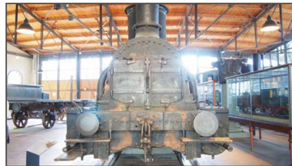
This locomotive was built in Austria. Its exterior bar frames are nearly 3 inches thick. It remained in service near Graz in Austria until 1960.
