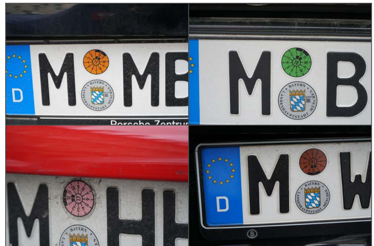
Photos show the Registration and Safety Seals on German License Plates. They indicate the schedule of regular safety checking of vehicle. Exhausted gas emission is also included as the criteria to pass the safety checking.
