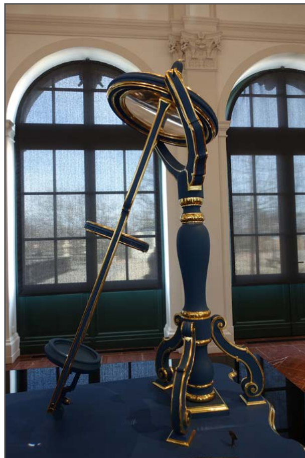
Double-lens Burning Apparatus by Ehrenfried Walther von Tschirnhaus in 1690
