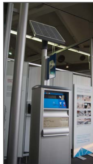
A photovoltaic powered automated payment machines for car parking
